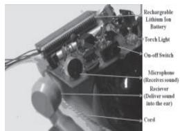
**Figure 6:** Indicating the different parts of the Low cost multi use hearing aid.
