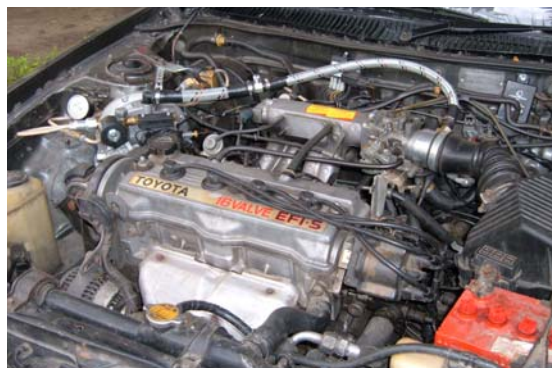
Fig. 2: CNG conversion components fitted on a typical automotive engine.
