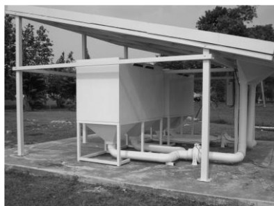
Figure 2. Photograph of the solar drying system with double-pass collector with fins.
