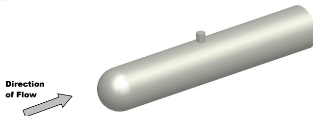
Fig. 1: Solid model of the hull-form with short H=D lateral pin-protuberance
