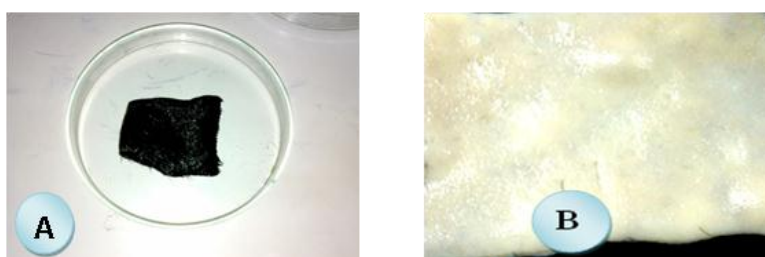
Figure 7. Direct dehairing activity of the enzyme - A is Control (Left) and B (100% Hair removed).
