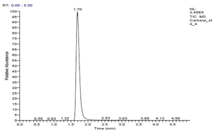
Figure 3. Chromatogram of carbaryl showing retention time.
