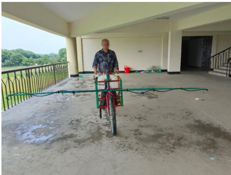
Fig. 8. Spraying coverage area measured on floor in the workshop.
