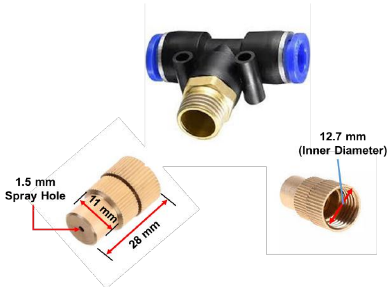
Fig. 3. Spray nozzle and its dimensions.
