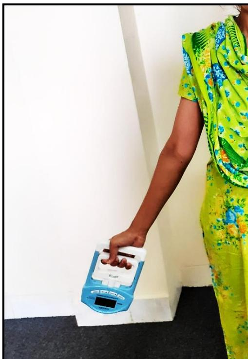
**Figure 1. Procedure of measuring the dominant handgrip strength using digital handgrip dynamometer.**
