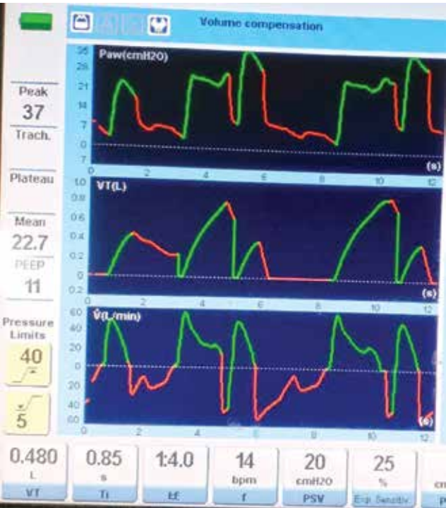
Figure 14: Multiple asynchrony present. Delayed termination 2, Double-triggering 2 & Ineffective triggering 2.
