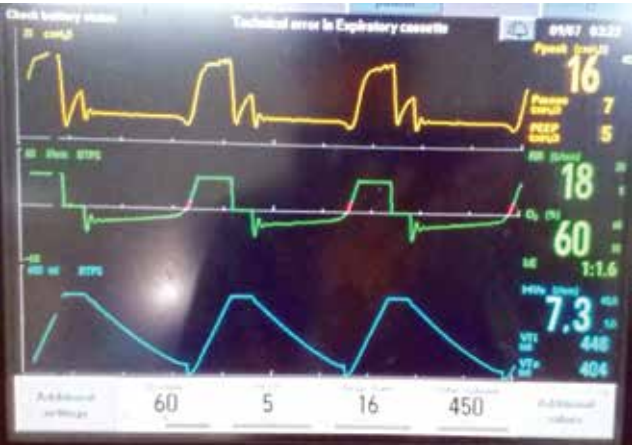
Figure 13: All three breath shows premature termination.
