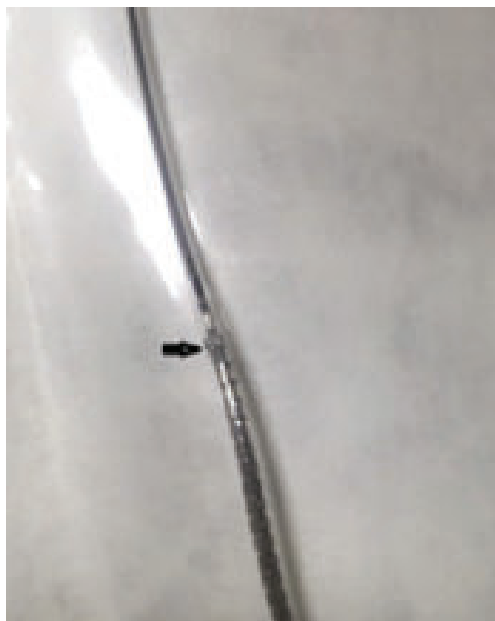
Fig.-2: Zoomed in view of distal end of stent balloon showing stent strut fracture (arrow).
