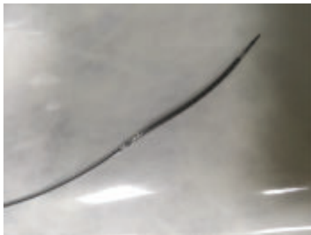
Fig.-1: Image shows the deformed distal end of stent balloon showing stent strut fracture
