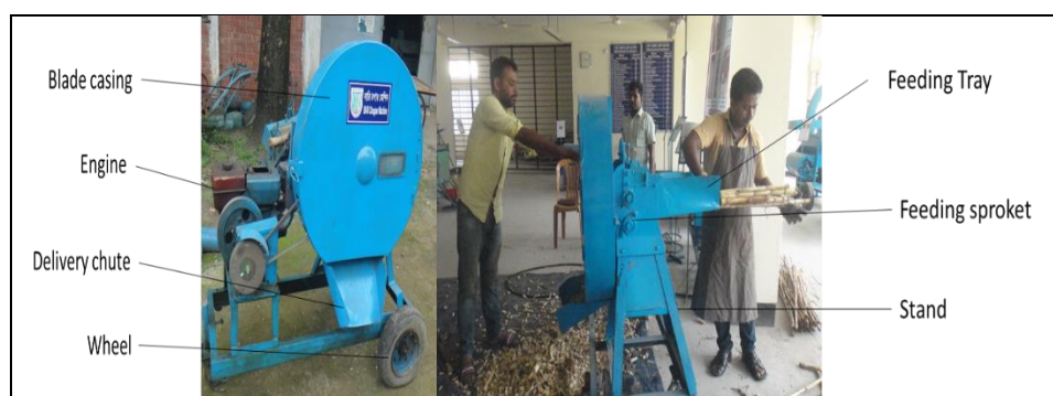
Fig. 1. Operation of BARI chopper for chopping maize stalk
