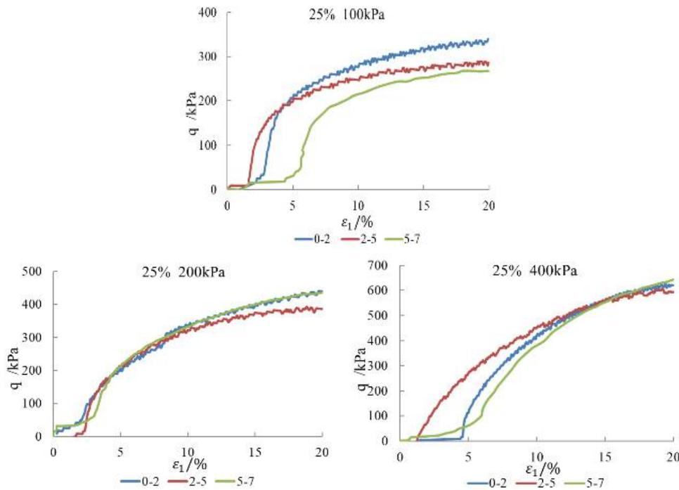
Fig. 10. Stress-strain curves of different particle sizes under the same confining pressure.
