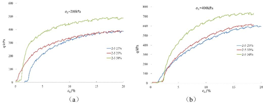
Fig. 8. Stress-strain curves of different contents under the same confining pressure.
