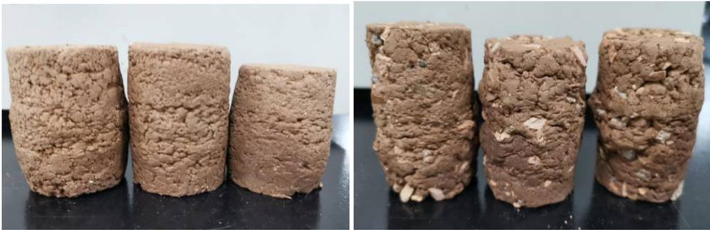
Fig. 7. Influence of different particle size and confining pressure on soil failure mode.
