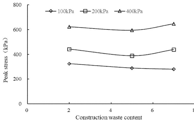
Fig. 9. Relation curve between peak deviatoric stress and construction waste content.
