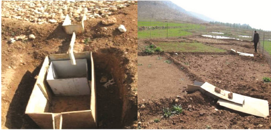
Fig.5. Stone Cover and Surface Compaction Runoff and Sediment Measurement System (Kuzucu 2013).
