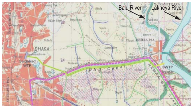
Figure 1. Raw water source and its transmission network from Lakheya River through DND canal to SWTP.
