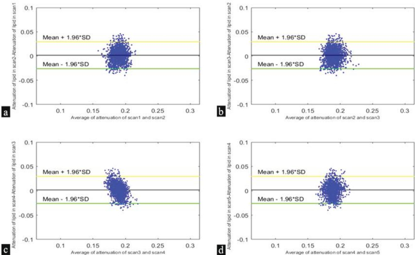
**Fig. 11.** Bland-Altman plot of single material such as lipid (a) for scan 1 and scan 2 (b) for scan 2 and scan 3 (c) for scan 3 and scan 4 (d) for scan 4 and scan 5 at lower energy bin. There are significant measurement points outside the limit of agreement.
