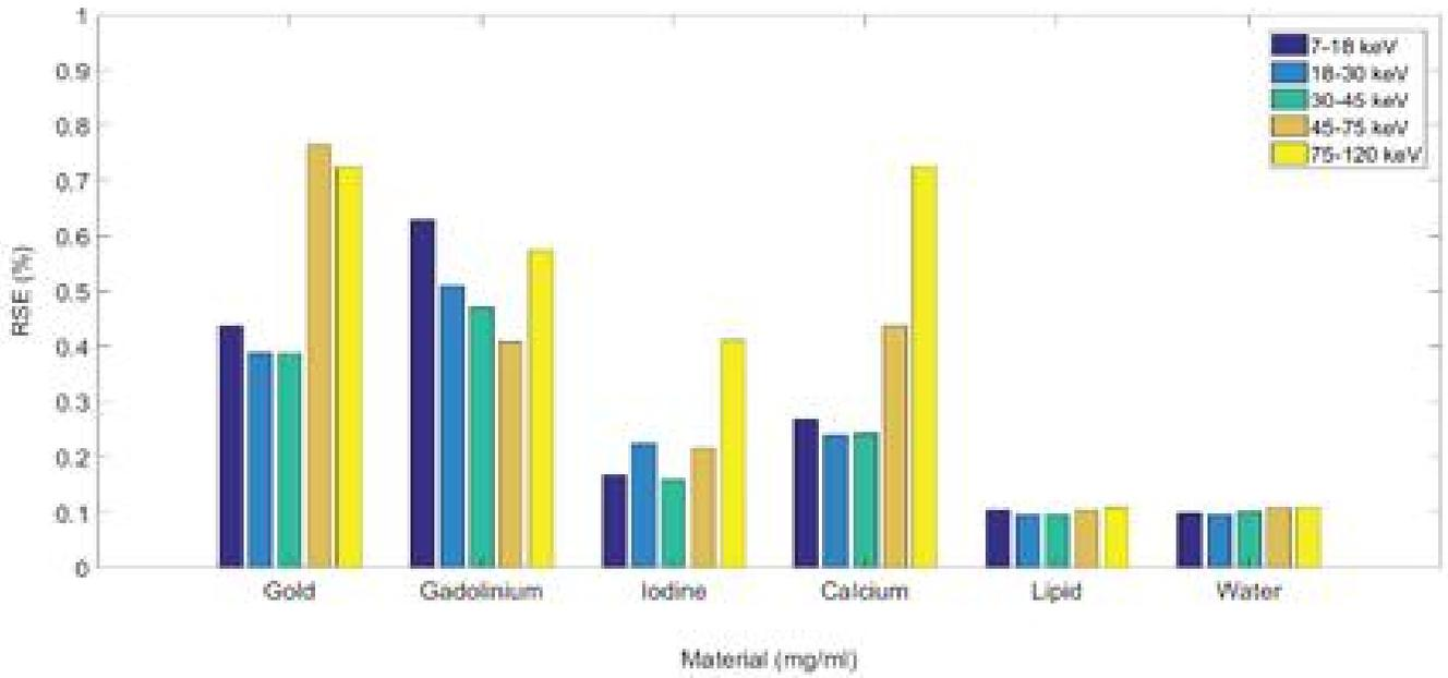
**Fig. 8.** The intra-scan variation of mass attenuation coefficient of different materials at different energy bins within any particular scan. Fourth and fifth energy bins show the higher value of RSE of gold, gadolinium, iodine, and calcium than lipid and water.
