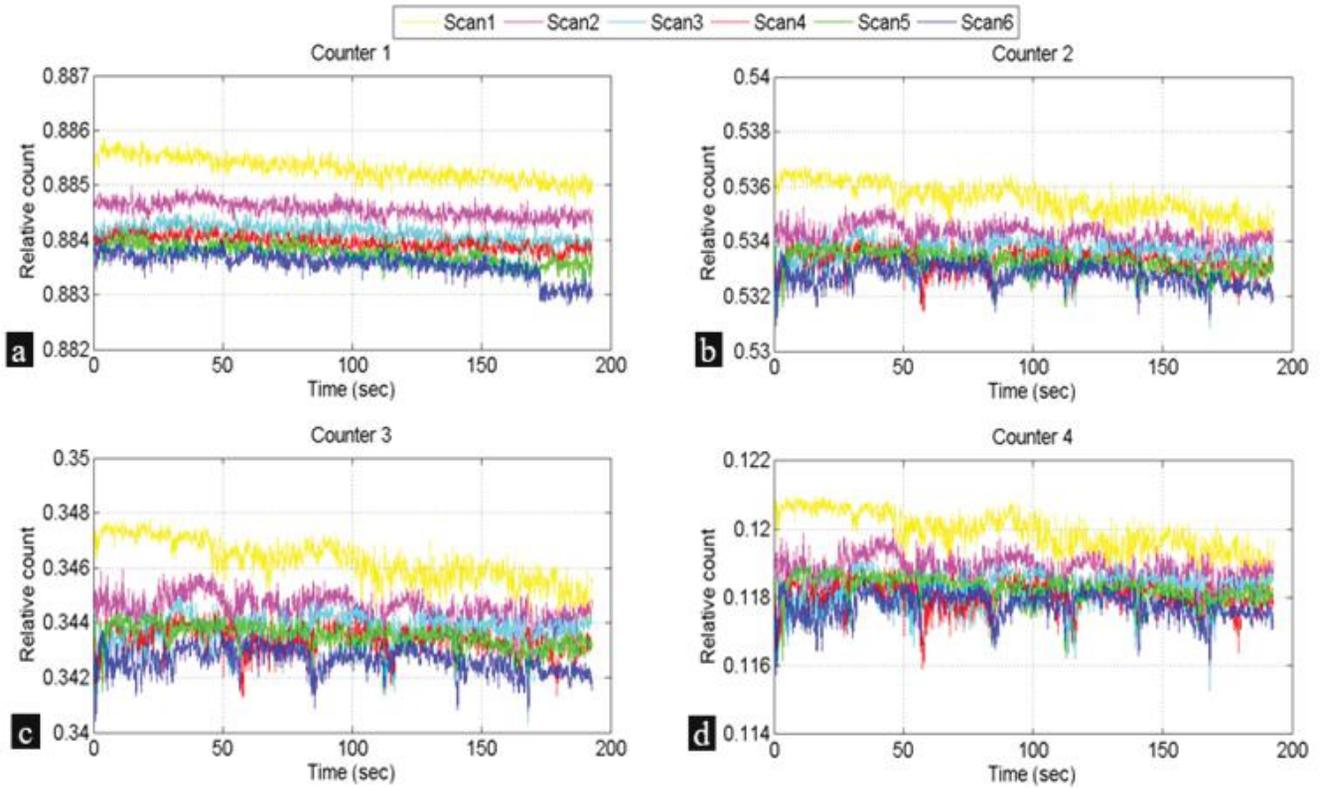
**Fig. 13.** The relative count in each scan of the different counter (a) first charge summing counter (b) second charge summing counter (c) third charge summing counter (d) fourth charge summing counter. The variation in the ASIC temperature could be the possible reason for the variation in counts with time.
