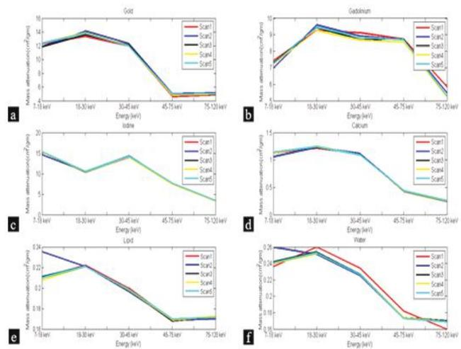
**Fig. 7.** Mass attenuation profiles (a) for gold (b) for gadolinium (c) for iodine (d) for calcium (e) lipid and (f) for water that used multi-contrast phantom with CZT-Medipix3RX detector at different energy bins of repeated scans. Mass attenuation value of lipid and water in scan-2 is slightly higher at 7-18 KeV but scan-1 is far from than other scans in case of water.
