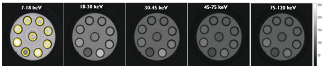
**Fig. 4.** Reconstructed images of a multi-contrast phantom obtained by MARS scanner with CZT-Medipix3RX detector in five energy bins. In the first image from the left, selected ROIs are also demonstrated.
