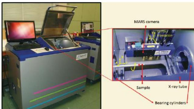
**Fig. 1.** A small-bore MARS spectral CT scanner. The magnified image (right) shows the x-ray tube, camera, and sample inside the gantry. The x-ray source and camera are mounted on the gantry that rotates around the subject.
