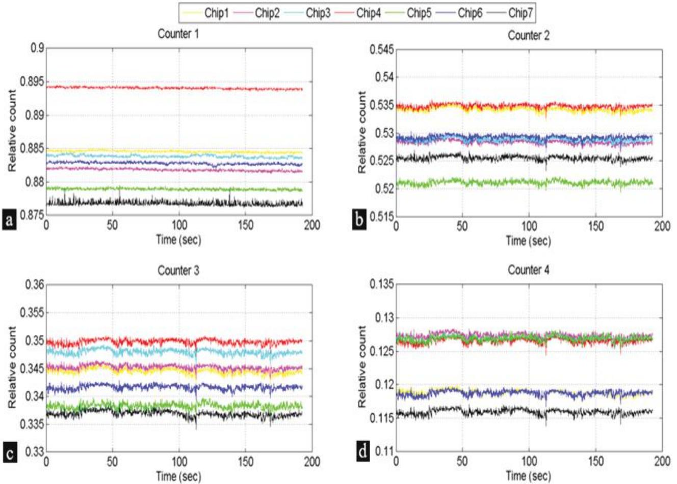
**Fig. 12.** The relative count rate of the different (CSM) counters (a) first charge summing counter (b) second charge summing counter (c) third charge summing counter (d) fourth charge summing counter with respect to arbitration counter in each chip during the initial scan.
