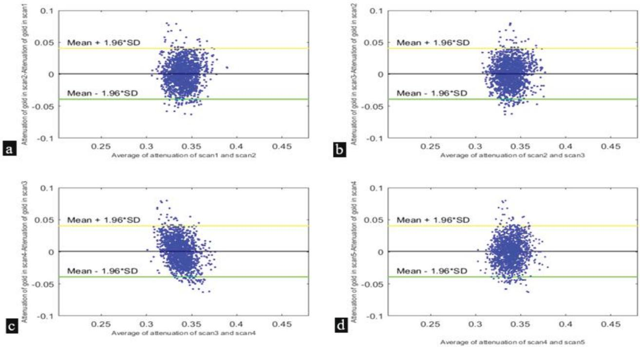
**Fig. 10.** Bland-Altman plot of composite material such as gold (a) for scan 1 and scan 2 (b) for scan 2 and scan 3 (c) for scan 3 and scan 4 (d) for scan 4 and scan 5 at lower energy bin. There are significant measurement points outside the limit of agreement.
