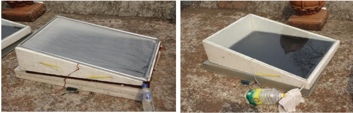
Figure 1: Basin type solar still with transparent PVC sheet cover (left) and glass sheet cover (right).
