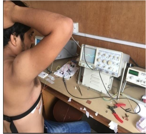
Figure 7. Electrode set up for measurement of impedance under breathe-in and breathe-out conditions
