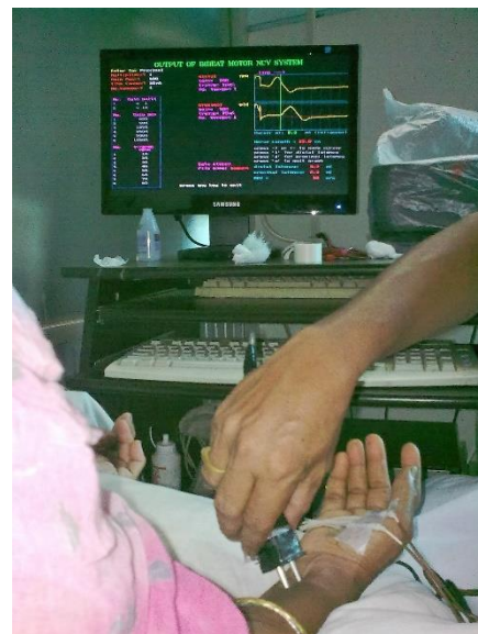
Fig.3. EMG/EP equipment based on a IBM compatible PC. Photo shows its use in nerve conduction investigation.
