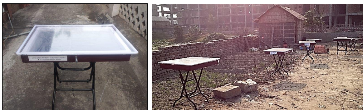
Fig 10: Enhanced model of solar water Pasteuriser using packing foam (polystyrene foam), black cloth as a base, water in transparent polythene bag and covered by two polythene sheets wrapped around a frame of PVC pipe (left). Residents of an urban slum using these devices as a normal routine (right).
