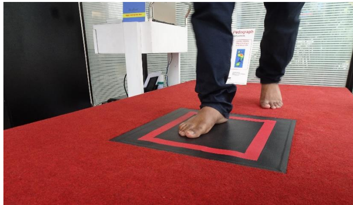
Fig 13: Top surface of the Dynamic Pedograph made by the author’s group. The marked region (the black region within the red marked tape) is the sensitive area and a patient walks with a foot onto this to give a scanned image.
