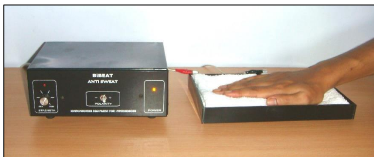
Fig.5: Iontophoresis equipment for treatment of Hyperhidrosis (excessive sweating of palms and soles)
