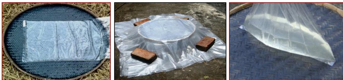
Fig 9: Solar water Pasteuriser using blackened bamboo tray on a thick bed of hay, water in transparent polythene bag and covered by two polythene sheets with air gap in between. This makes a flat plate collector that utilizes 'Green House Effect'. Heated water harvested in the bag.
