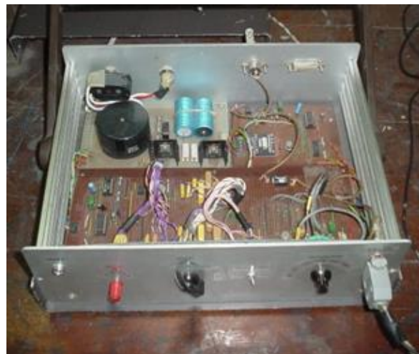
Fig.2: Inside of a second unit of EMG/EP equipment which the author's group made indigenously later in Bangladesh.
