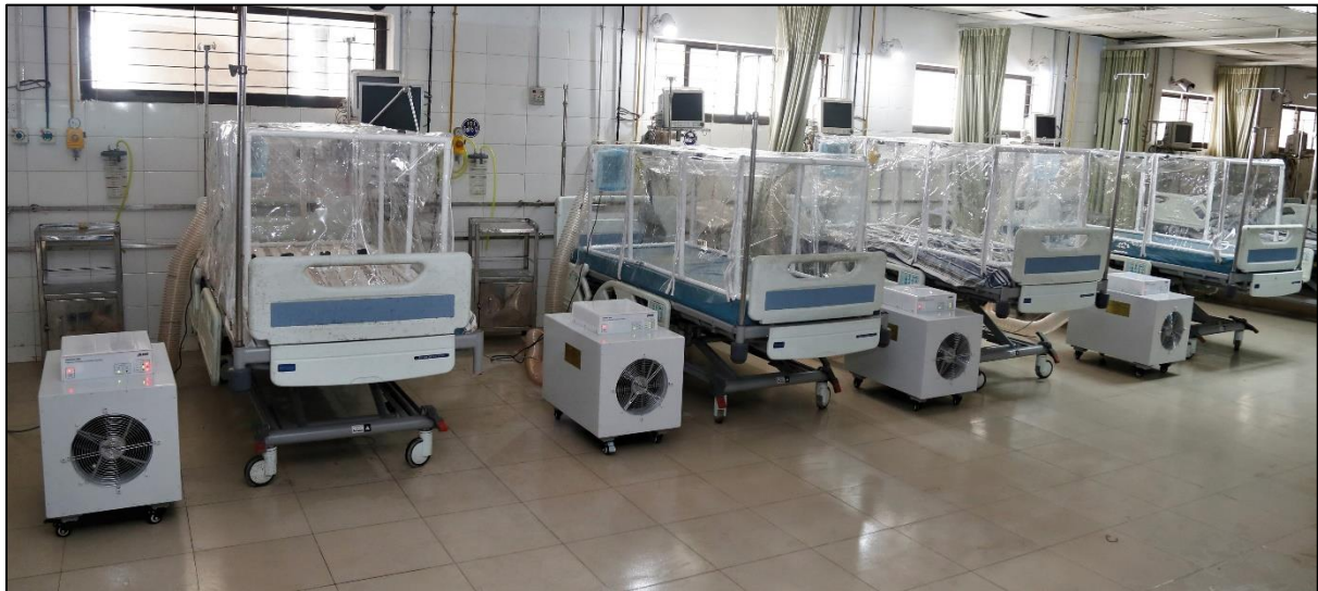
Figure 19. Negative Pressure Isolation Canopies, designed and developed by the author's group, installed at BSMMU, Dhaka
