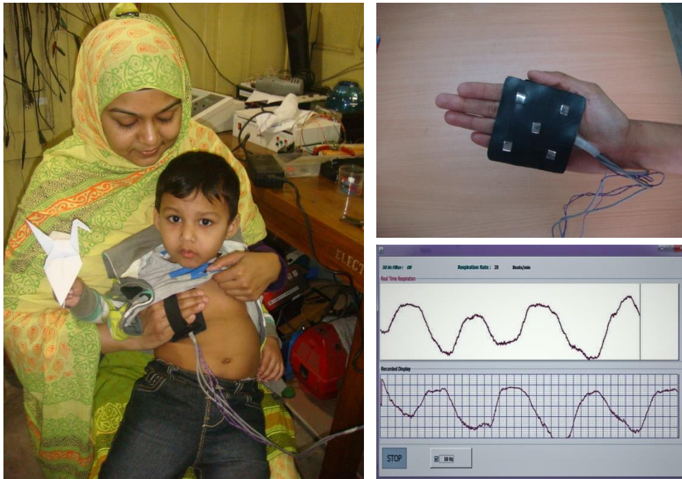
Fig 15: A mother holds a palm-worn four electrode FIM probe (fifth electrode for ground, eliminated later) on her child to get the tidal breathing waveform from which necessary lung ventilation information including breathing rate can be obtained. The interesting part is that the child did not cry during the procedure, which would have jeopardised the whole effort since crying changes breathing rate [93]
