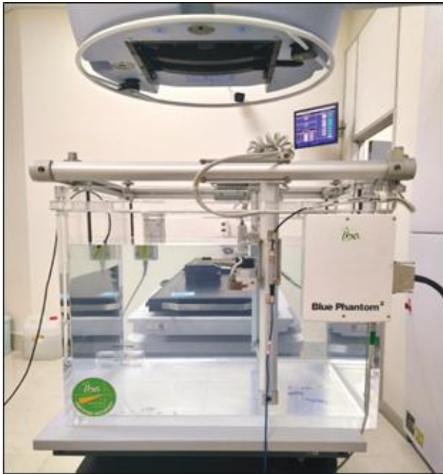
Fig. 1: Pictorial representation of measurement of absorbed dose rate to water using a Farmer chamber at SSDL, BAEC, Savar, Dhaka, Bangladesh.
