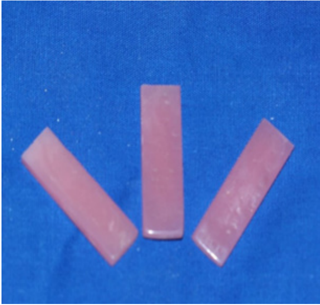
Figure 3. Acrylic bars for testing flexural strength (60mm×10mm×3.3mm)
