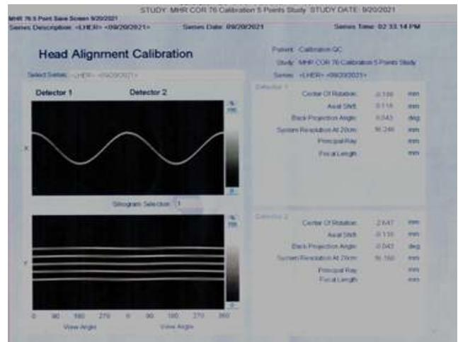
**Figure 3: COR test for 180, 90, 76 degrees angle configuration**
