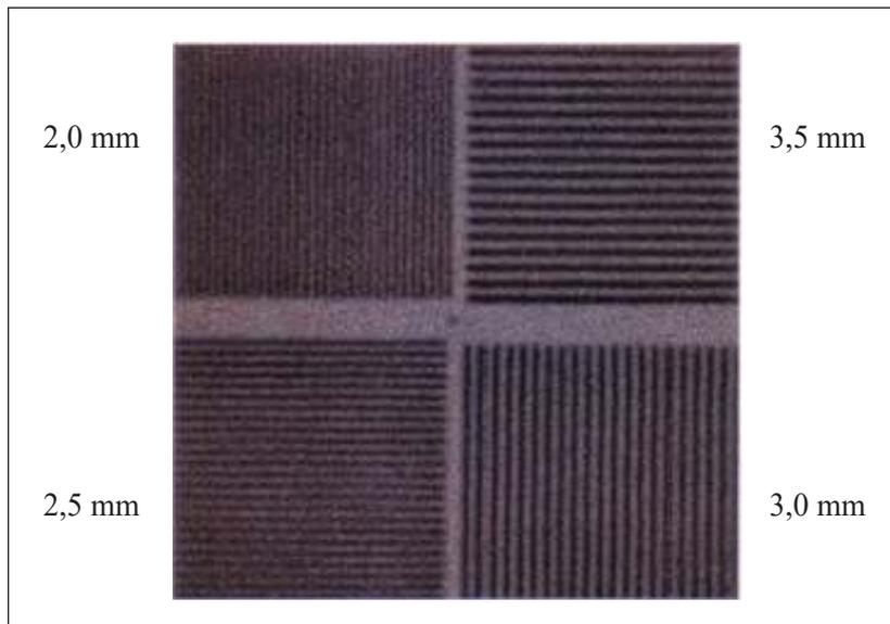
Figure 8: Resolution by using bar phantom
