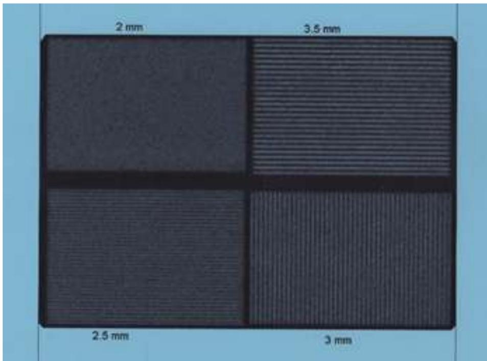
Figure 4: Resolution by using bar phantom
