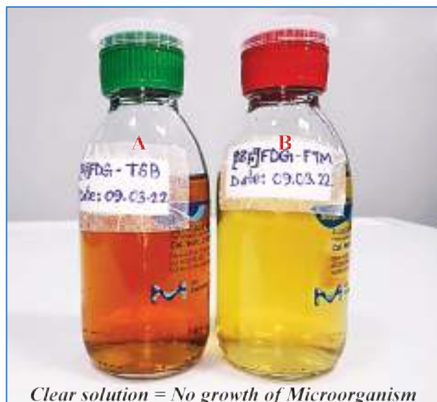
Figure 6: Sterility test of the final [ ^{18}\text{F} ]FDG product, (A) TSB media incubated at 22.5°C (B) FTM media incubated at 32.5°C for 14 days.
