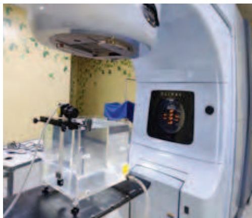
Figure 1: Experimental setup of ionization chamber set in 1D water phantom
