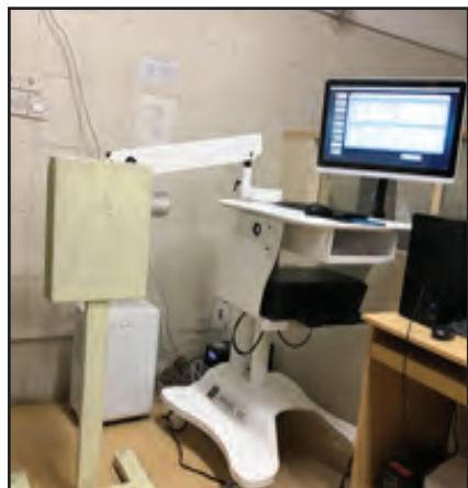
Figure 7: Folded Lead Barrier for I-131 Uptake Injection
