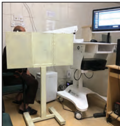
Figure 8: Unfolded Lead Barrier for ^{131}\text{I} Uptake Machine
