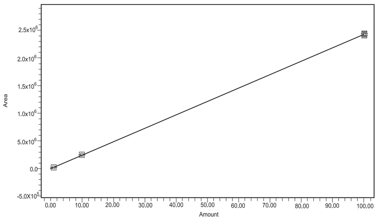
Name: Amoxicillin; RT: 3.442; Fit Type: Linear (1st Order); Cal Curve Id: 4817; R:0.999998; R<sup>2</sup>: 0.999995; Weighting: none; Equation:  $Y = 2.44e+004 X + 3.28e+003$
