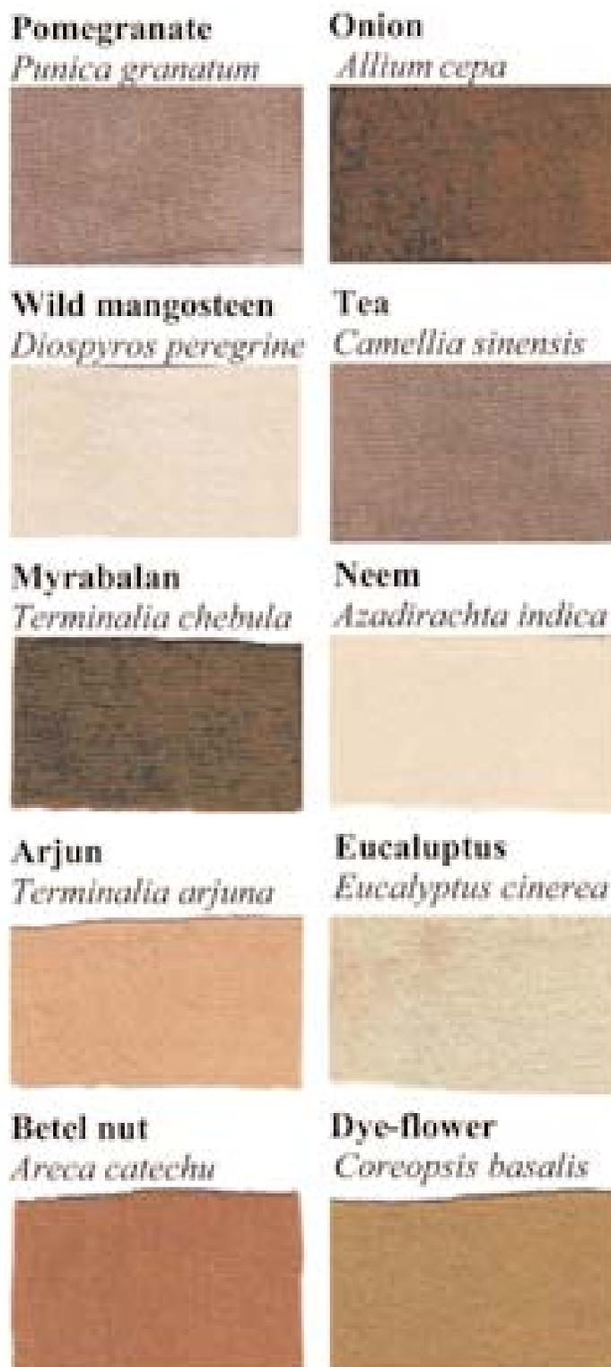
Fig. 1. The corresponding colour of cotton (100%) fabrics obtained from dyeing with different plant materials after checking wash fastness
