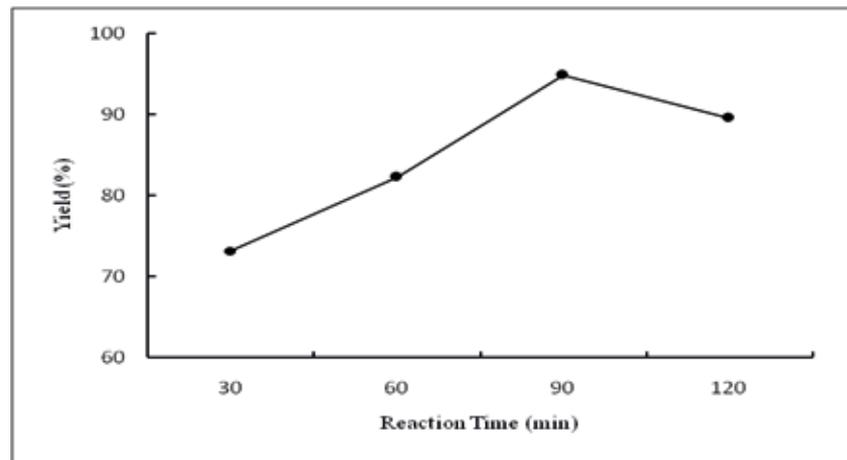
Fig. 5. Effect of reaction time on bio-lubricating base oil yield
