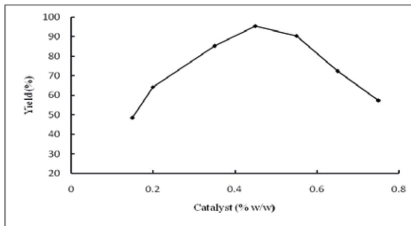
Fig. 3. Effect of catalyst concentration on bio-lubricating base oil yield
