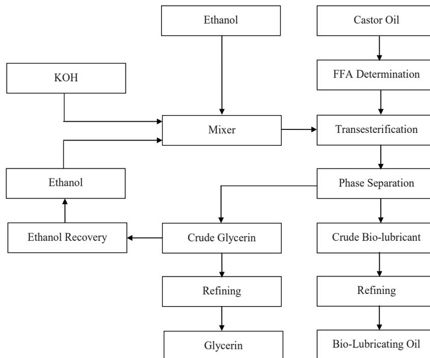
Fig. 1. Flow diagram of bio-lubricating base oil production from castor oil
