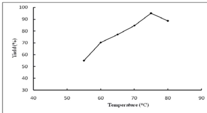
Fig. 4. Effect of temperature on bio-lubricating base oil yield
