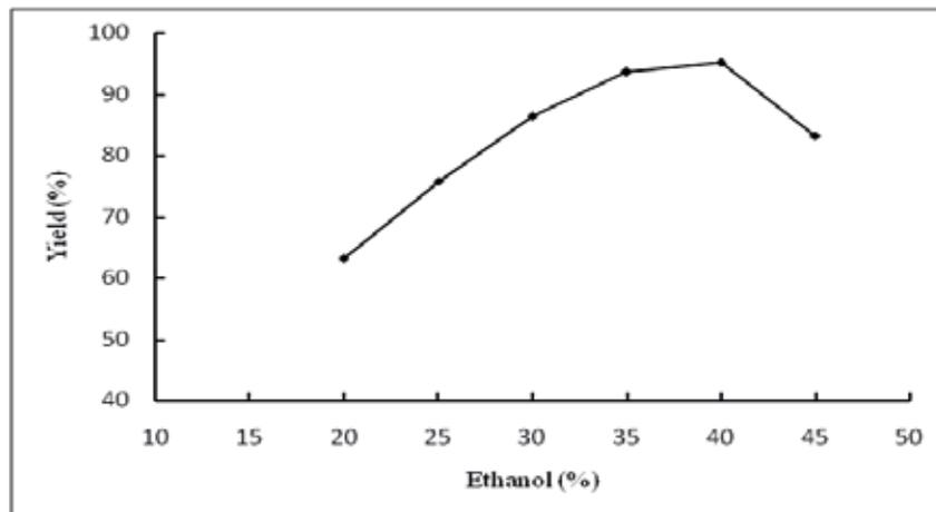
Fig. 2. Effect of ethanol percent on bio-lubricating base oil yield
