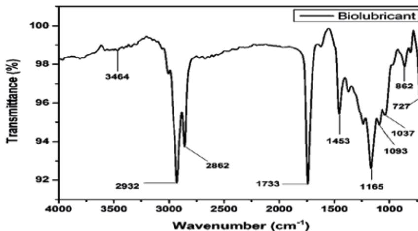
Fig. 6. FTIR spectra of bio-lubricating base oil
