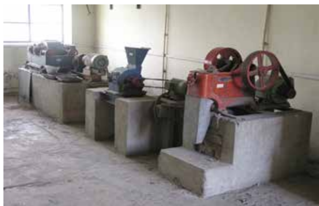
Fig. 1(b). Laboratory scale jaw crusher and roll crusher used for sample preparation
