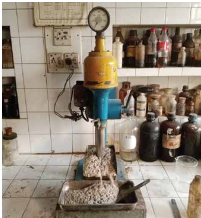
Fig. 1(c). Denver D-12 flotation machine used for flotation of fluorite ore
