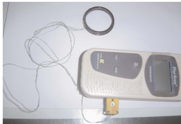
Fig. 6. Measurement of ring temperature by K type thermocouple system
