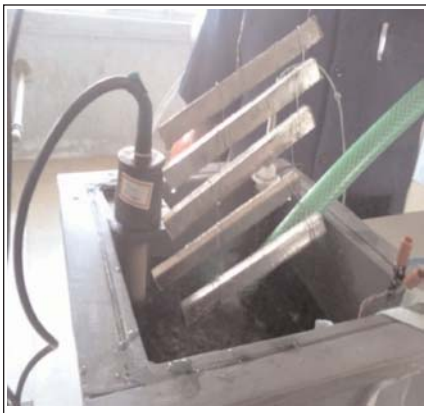
Fig. 8a. Nickel plating tub with solution (nickel plated flexure specimen also visible)
