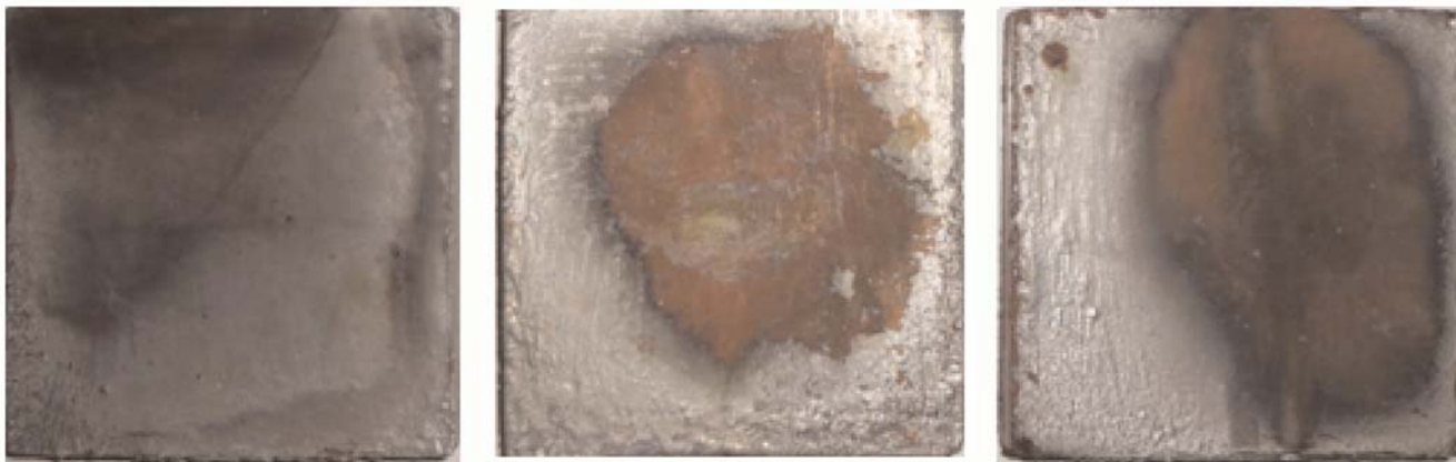
Fig. 14. Variation in electroplating parameters cause uneven plating
