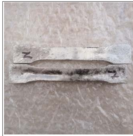
Fig. 8b. Nickel plated tensile specimens
