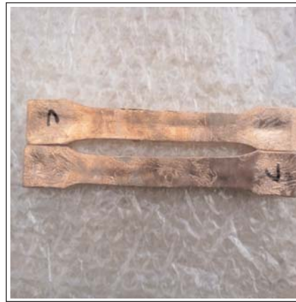
Fig. 7b. Copper plated tensile specimens
