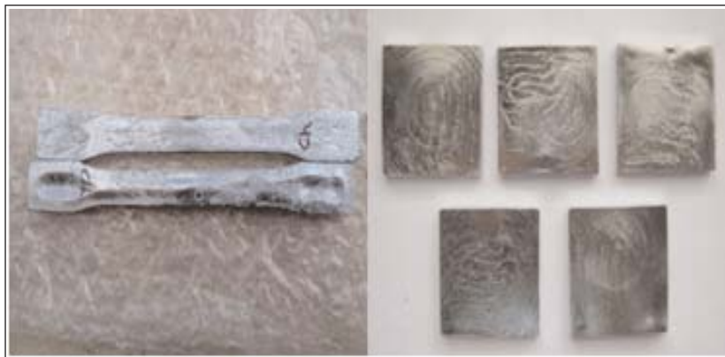
Fig. 9. Chrome flashed tensile and hardness samples
