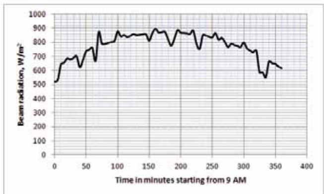
Fig. 4. Beam radiation intensity falling on the reflectors from 9:00 AM to 3:00 PM.
