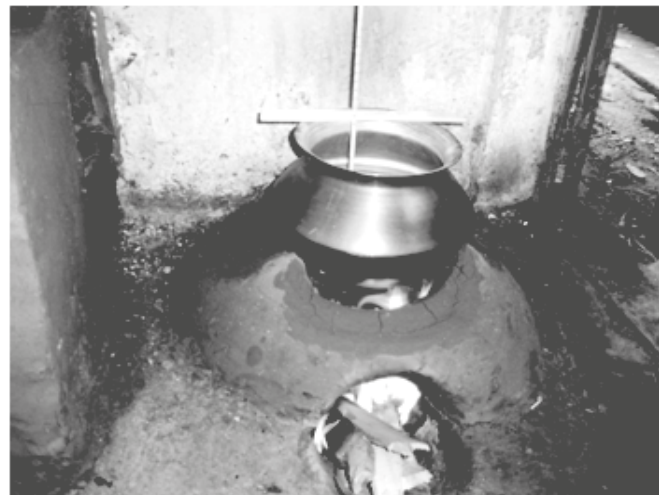
Fig. 2. Traditional single mouth underground stove used in Bangladesh which is made of clay and without grate.
