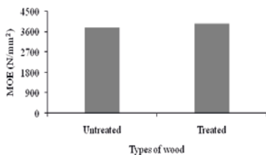
Fig. 6. Effect of CCB preservative treatment on MOE of A. richardiana wood
