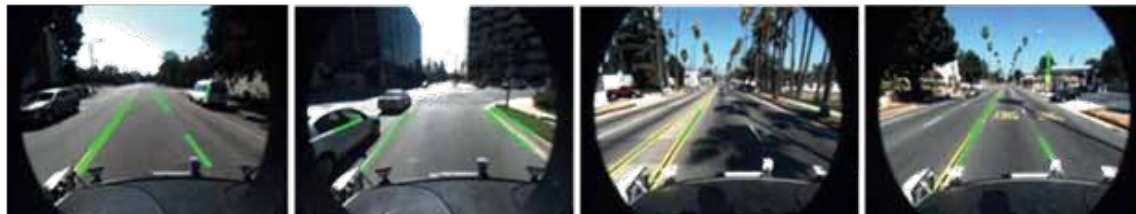
Fig. 10. False detection samples result. (a) is related to the Cordova 1 database and edge of the car misdiagnosed. (b) is related to the Cordova 2 database and edge of the car misdiagnosed. (c) is related to the Washington 1 database and not a complete diagnosis. (d) is related to the Washington 2 database and object along the street is misdiagnosed.
