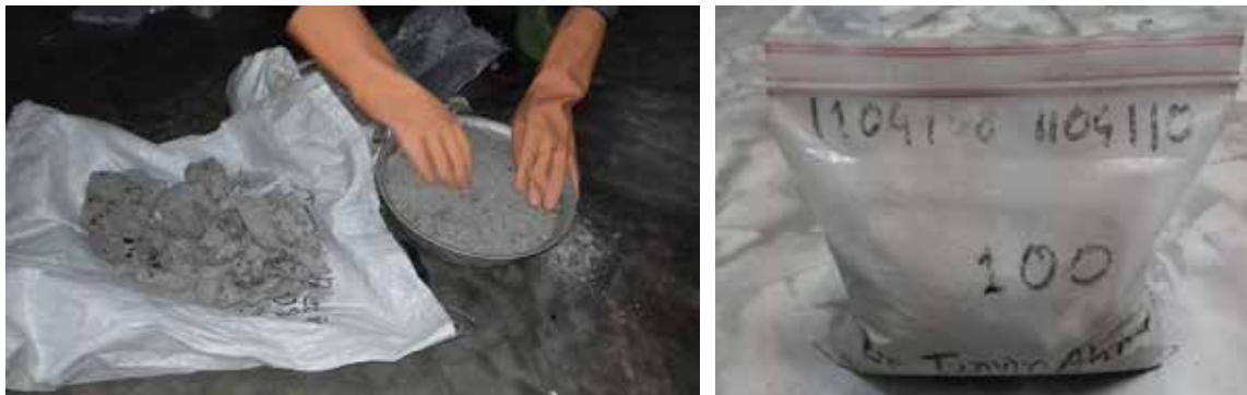
Fig. 2. Separation of large particles from incineration fly ash manually and storage of the prepared sample in zip-lock bags
