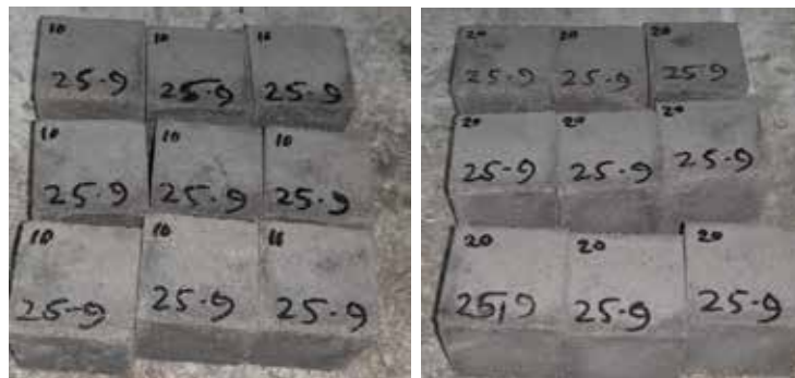
Fig. 3. Cement-mortar cube specimens consisting of 10% and 20% fly ash
