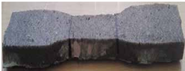
Fig. 1. Fabricated composite D (FG: resin: hardener = 60:50:25) at optimized conditions
