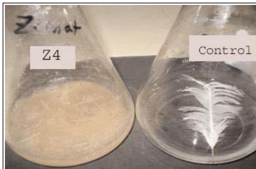
Fig. 3. A representative illustration of feather degradation by the most potent keratinolytic isolate Bacillus Z4
