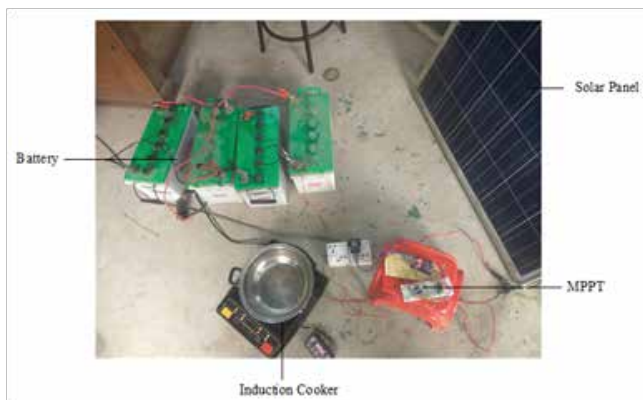
Fig. 14. Experimental setup of induction cooker
