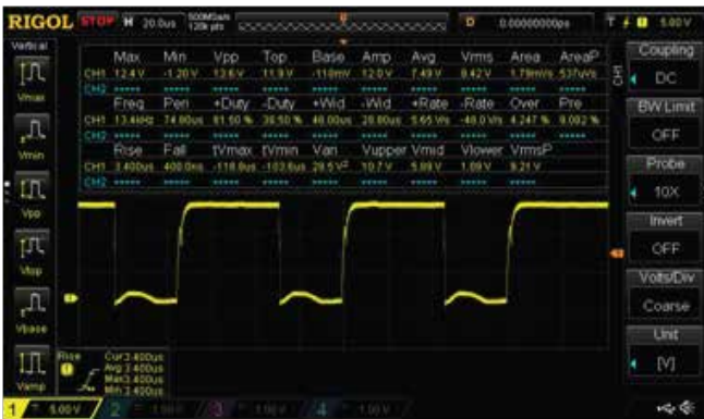
Fig. 17. IGBT gate voltage waveform at power level 6
