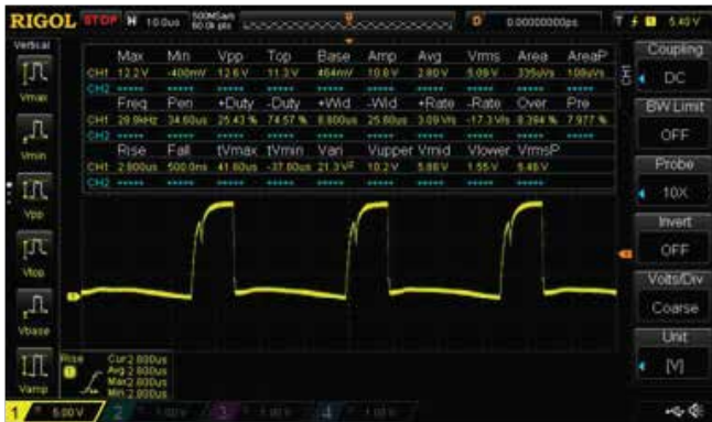
Fig. 16. IGBT gate voltage waveform at power level 1
