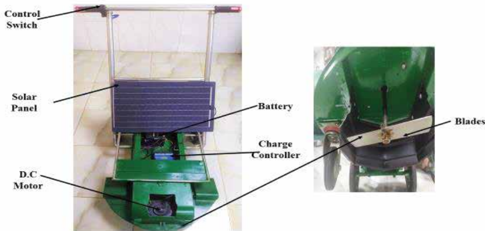
Fig. 7. Different components of solar grass cutter used in this project
