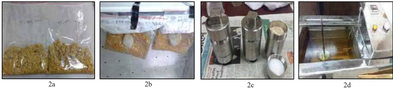
**Fig. 2. a) 20-40 mesh size SB and alkali were taking into plastic zipper bag; b) samples were pretreated into water bath at a temperature below 100°C; c) 20-40 mesh size SB and alkali were taking into stainless-steel reactor; d) sample pretreated into oil bath at a temperature above 100°C**
