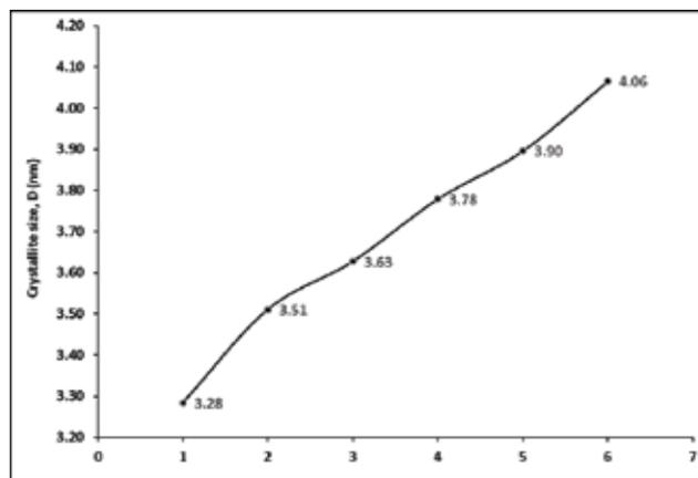
**Fig. 5. Average size of crystalline for raw SB, 0, 2, 4, 6 and 8% alkali treated sample**
