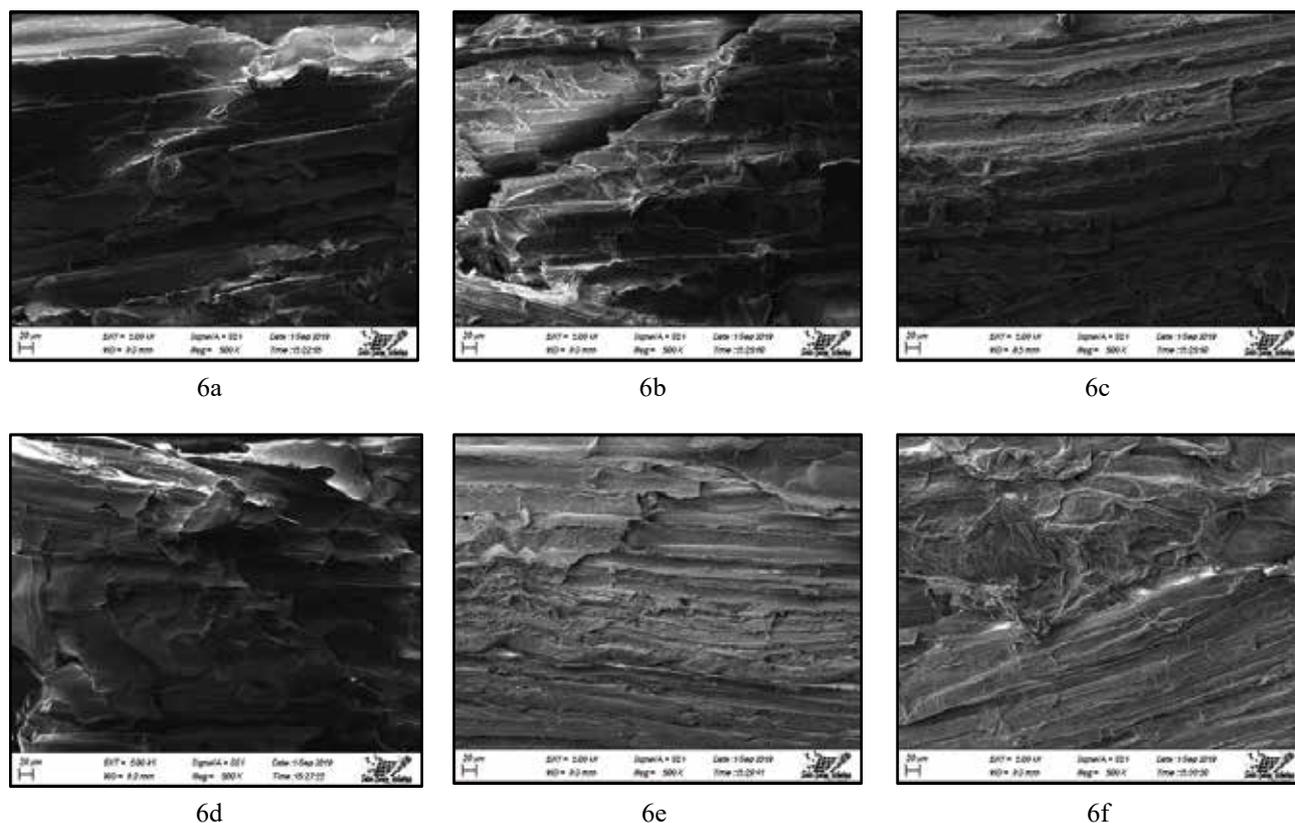
Fig. 6(a-f). SEM images a) 20-40 mesh size SB; b) 0% alkali treated sample; c) 2% alkali treated sample; d) 4% alkali treated sample; e) 6% alkali treated sample; f) 8% alkali treated sample
