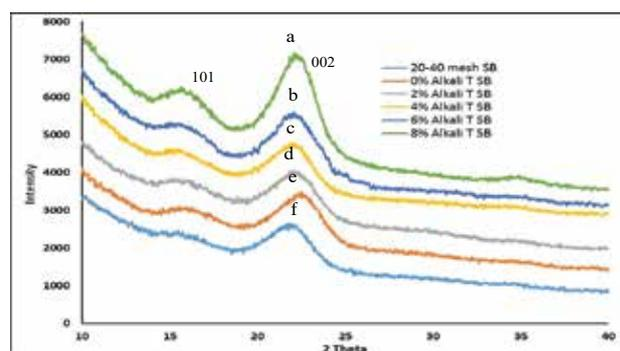
**Fig. 4. XRD spectra of a) 20-40 mesh size SB; b) 0% alkali treated sample; c) 2% alkali treated sample; d) 4% alkali treated sample; e) 6% alkali treated sample; f) 8% alkali treated sample**
