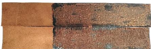
Fig. 6. Peel strength test for prepared bio –adhesives
