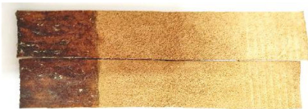
Fig. 5. Shear strength test for prepared bio-adhesives
