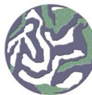
Figure 3: Schematic showing iron oxide filling media cracks and crevasses
