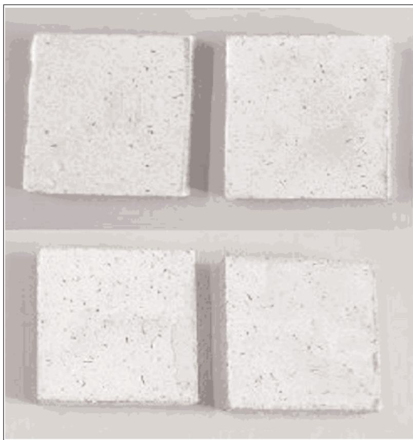
Fig. 1: Photograph of RHA- \text{TiO}_2 (top - 25% \text{TiO}_2 , bottom - 50% \text{TiO}_2 ) composite
