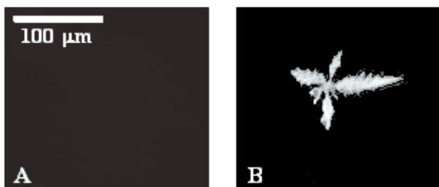
Fig. 5: BAM images of the Langmuir monolayers of NHEA-14 observed in situ during compression at 10 °C at different areas; (A) 0.6 nm 2 /molecule (B) 0.41 nm 2 /molecule
