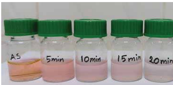
Fig. 4. Dye decolorization in different photo catalyst material ratio with visual representation
