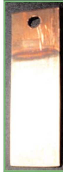
Fig. 1. Uniform, adherent and bright coating obtained from bath C-1
