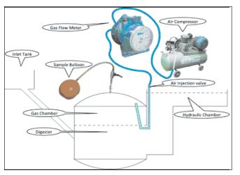
Fig. 1: Aeration arrangement for H<sub>2</sub>S reduction
