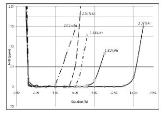
Graph 4: Duration of below desired level of H<sub>2</sub>S by aeration with different percentage of air
