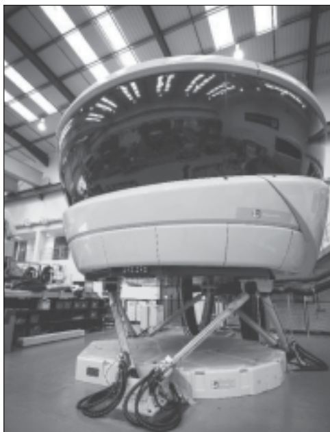
Fig.-9: The brand new Boeing 777 full-flight simulator (FFS) is being manufactured by L-3 Link Simulation & Training UK (L-3 Link UK) at its Crawley, UK facility.
