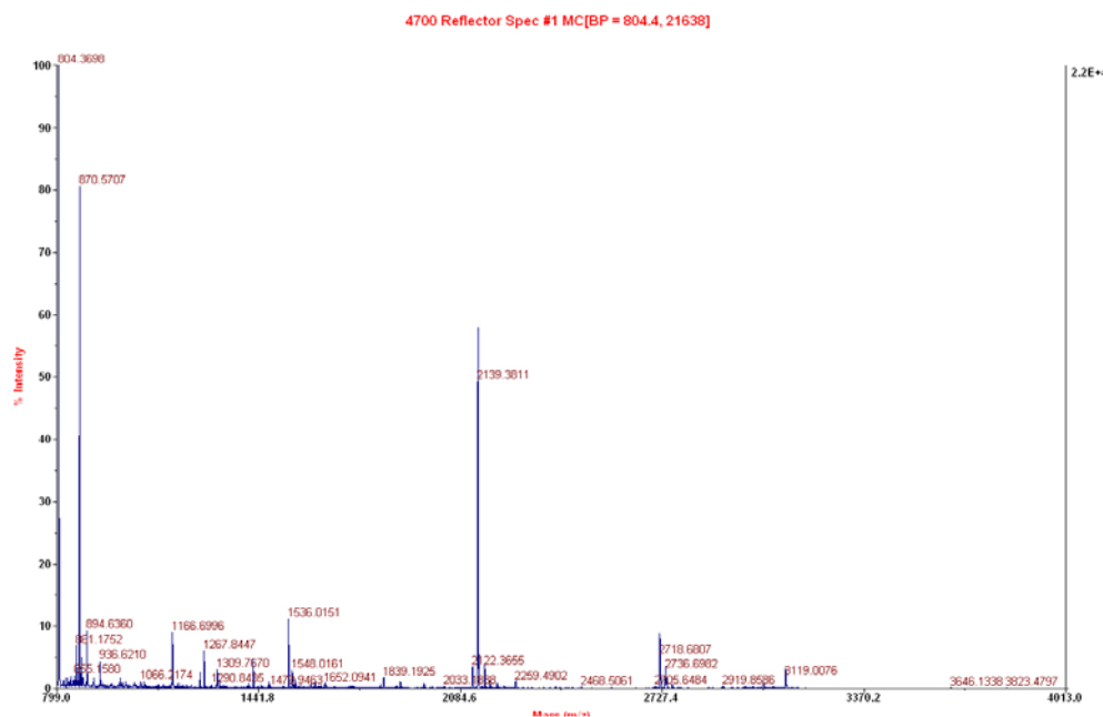
Fig. 8a. The mass spectrum showing peptide mass fingerprint (PMF) of ~17 kDa, recombinant aphrodisin protein band present in post-sonication pellets of IPTG induced cultures of BL21 cells. The peptide mixture was mass analyzed using AB4800 MALDI-TOF/TOF and the peptide masses were recorded as shown in the figure.
