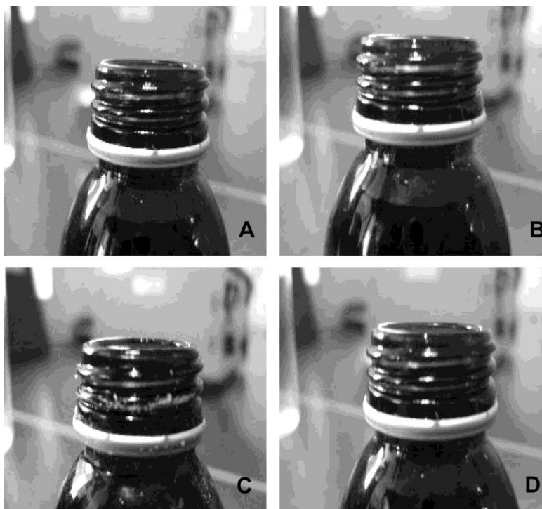
Figure 4. Photos representing crystal growth of DPH with sugar syrup & partially inverted sugar syrup spread inside cap and on bottle neck at zero time and after 2 weeks (at room temperature). A. DPH with sugar syrup (Control, P001) at zero time, B. DPH with inverted sugar syrup (Test, P002) at zero time, C. DPH with sugar syrup (Control, P001) after 2 week, D. DPH with inverted sugar syrup (Test, P002) after 2 week.
